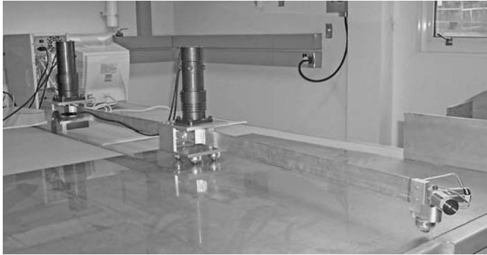
FIGURE 13.5 Prototype two-link flexible robot manipulator.
