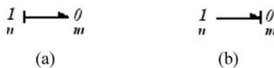
FIGURE 17.23 Connection of junctions: (a) connecting bond is not causality dominant, (b) connecting bond is causality dominant.
